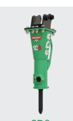
SD8 1 - 1.7 t Carriers 76.4 kg / 168 lb Operating Weight 15 - 30 l/min / 4 - 8 GPM Oil Flow
